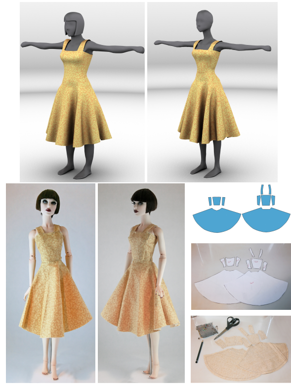
Figure 11: Validation on a real dress: we transferred the woman's dress on the top-left to a Numina doll model ©Dollcis (top-right) and used the patterns to make an outfit for the real doll (bottom). The virtual source and real graded patterns for the front and back of the dress at bottom right. ©Laurence Boissieux 2012
